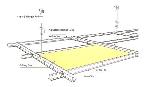
**Main Tee** is a double web section of 38 mm or 32mm high, made in standard length of 3.6 integral push lock splices at both ends for easy interconnection. The end splices have been tested to sustain a pulling force of 68kgf before separation. The bulb is pre-punched with "H" slots at 75mm from ends and 150mm in between to receive cross tees.
